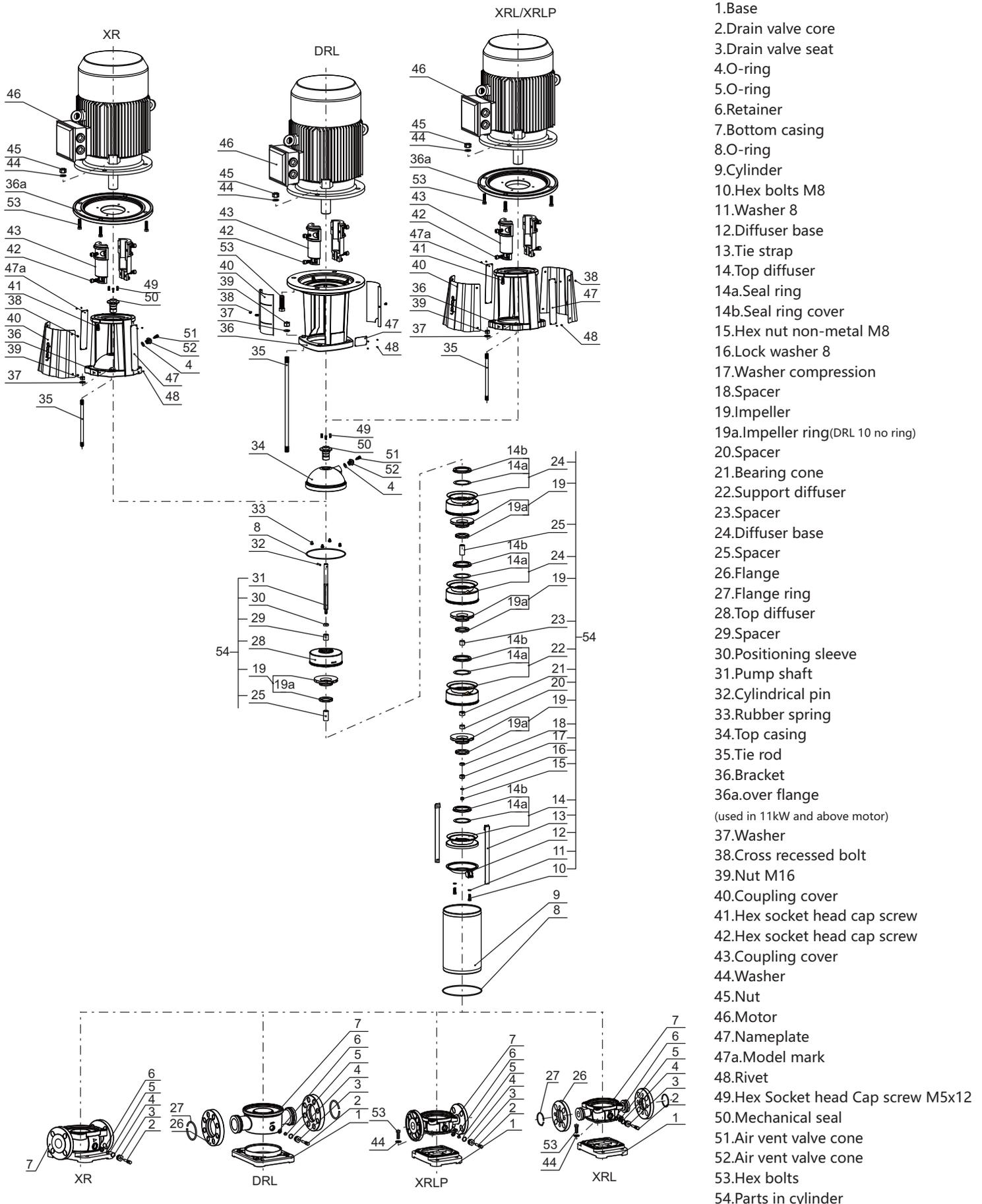
● 14 Picture 3 Exploded view for Model XR/DRL/XRL/XRLP 32~90
