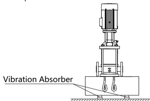
For motor power  $\geq 37\text{kW}$  as shown in the below picture, One Sylomer pad or Vibration pad recommended to use.
