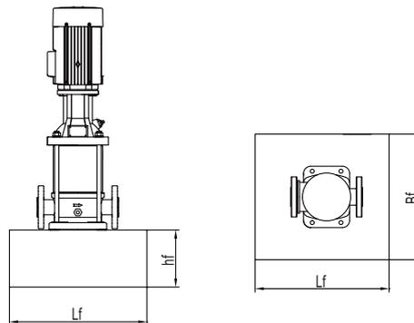
For the pump model whose motor power ≤30Kw, The length and width of foundation must be over 200 mm than the pump base. For the pump model whose motor power ≥37Kw, The length and width of foundation must be 1.5m X1.5m. The basic weight must be 1.5 times bigger than the total weight of the pump. The minimum height of the foundation can be calculated based on the concrete weight, density, and foundation length and width.
